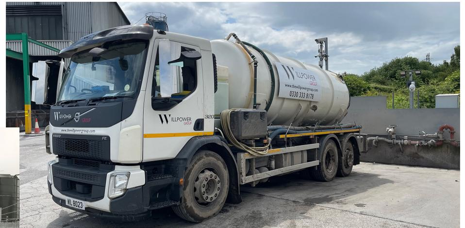
Our sewage tankers range from 500 gallons for restricted site access to 3000 or 4000 gallon lorries for larger waste removal needs. We also operate a JCB Fastrac and 3000 gallon tanker for muddy event sites or off road septic tank locations.
